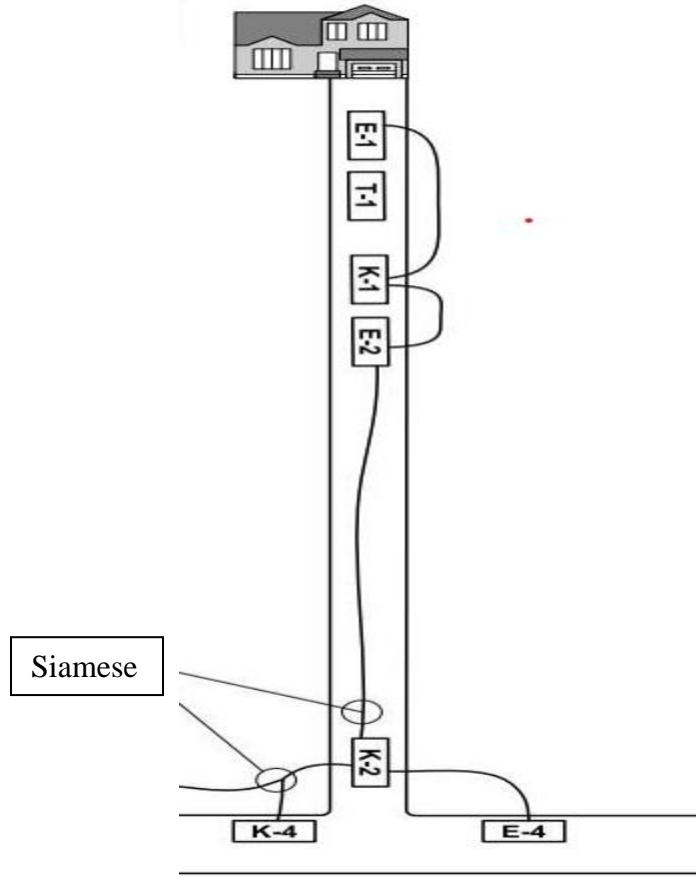
For long drive ways, additional apparatus can position for a relay operation.
