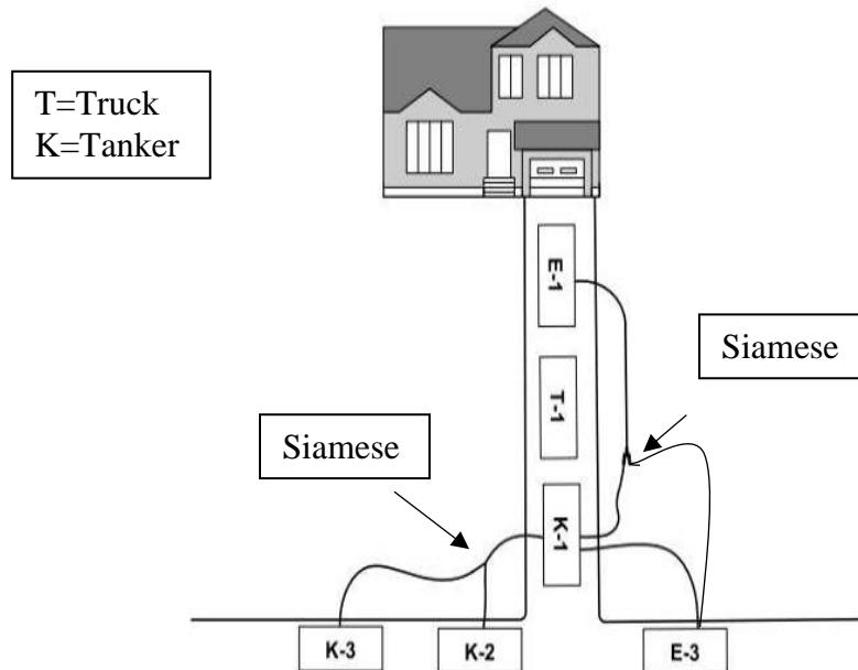
Direct Tank Fill Method (no drop tanks). 1<sup>st</sup> Tanker is committed to the scene.
